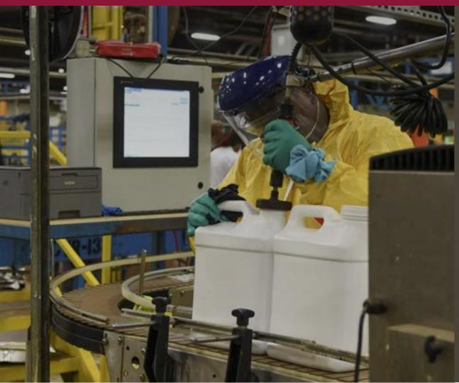
Single and multi-head filling lines packaging from 4 ounces to 5 gallons with bottom-up capability
