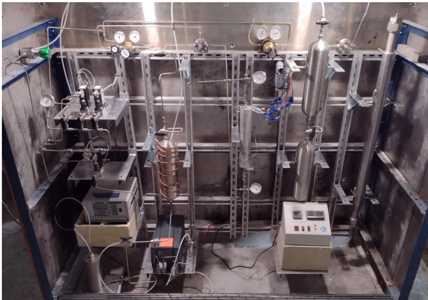
Lab scale continuous flow reactor with ½-in OD electrically heated reactor (center) and 1.5-in OD hot oil jacketed reactor (right). System rated to 1000 psig.
